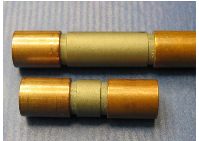
Cu rings as electrical contacts of ZrC products
